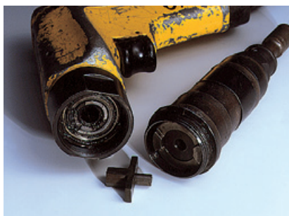
Damaged pneumatic tooling
